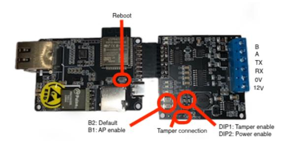
The onboard tamper connection can be enabled by disabling DIP1. This will enable the header pins and allow connection for an external tamper switch. The activation of the tamper switch results in the triggering of the tamper of a virtual keypad and is sent back to the panel and over MQTT as a device tamper.
