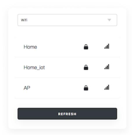
The Captive Portal allows for primary setup of either Wifi or Lan connection. Upon selection of the interface, a choice for DHCP or Static IP assignment is presented. After saving the settings, the portal will close. Manually restart the module to start the actual configuration. A web interface is presented to do this on the IP address the module has received from DHCP or the Statically assigned IP address.
